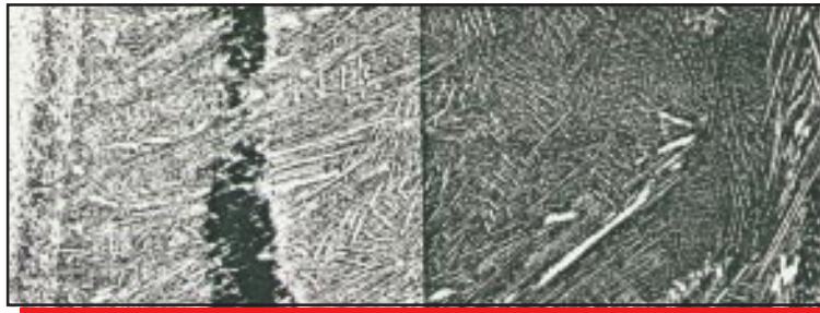
Top section of cupronickel, welded at 5 i.p.m. without vibration.
