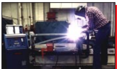
Meta-Lax Weld Conditioning of aluminum fixtures.
