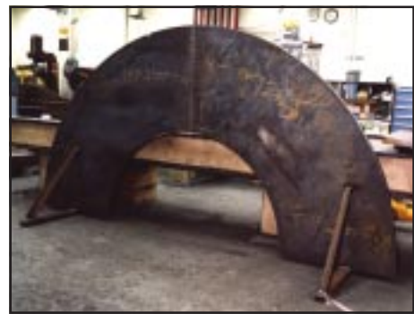
10 foot diameter disk after welding.
