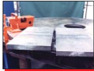
6061-T6 test plates after welding.
