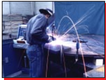
Meta-Lax Weld Conditioning of 6061-T6 test plates.
